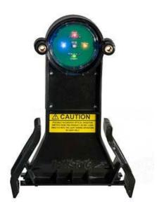
The colours are specially configured for you to tell a real image from a virtual. A real image is inverted (like a telescope) and a virtual image is upright (like a mirror). Inversion swops left with right and up with down, i.e. green with red, and blue with yellow, like so:
