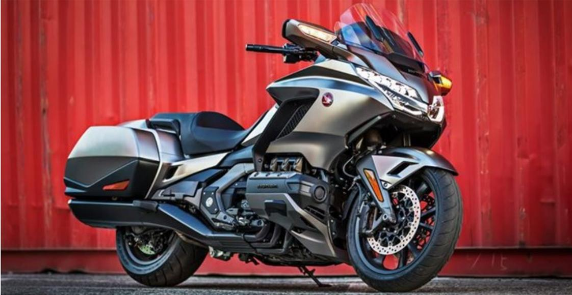
The new chassis features an aluminium beam frame, double wishbone front suspension and single-sided Pro-Arm – damping is electrically adjustable, as is rear spring preload. An electric screen, Smart Key and Apple CarPlay are also standard equipment. An entirely new, third generation of Honda's dual clutch transmission (DCT) - with seven speeds - will also be available.
