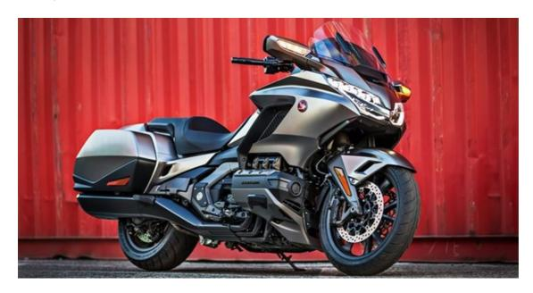
The new chassis features an aluminium beam frame, double wishbone front suspension and single-sided Pro-Arm – damping is electrically adjustable, as is rear spring preload. An electric screen, Smart Key and Apple CarPlay are also standard equipment. An entirely new, third generation of Honda's dual clutch transmission (DCT) - with seven speeds - will also be available.
